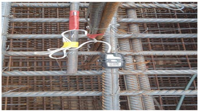
Global Lab has the experties to evaluate the compressive strength of concrete using Maturity method.
