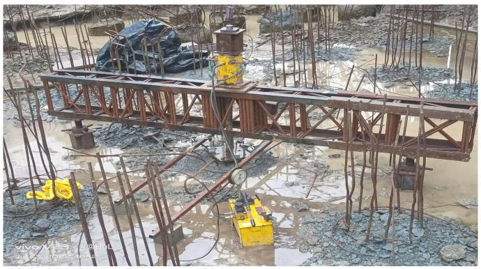
Global Lab has the Pile Pullout Testing facility upto 100T as per IS 2911 Part-4 under scope of NABL.
