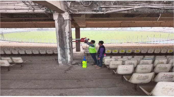
Global Lab offers the precise, accurate & reliable Concrete core testing accredited by NABL complying the requirement of IS 516 & IS 516 Part-04.
