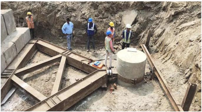
Global Lab has the Pile Lateral Load Testing facility upto 100T as per IS 2911 Part-4 under scope of NABL.
