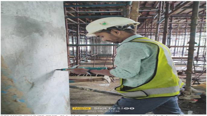
REBOUND HAMMER TEST: Global Lab offers the precise, accurate & reliable Rebound Hammer testing accredited by NABL complying the requirement of IS 13311 Part-2: 1992.
