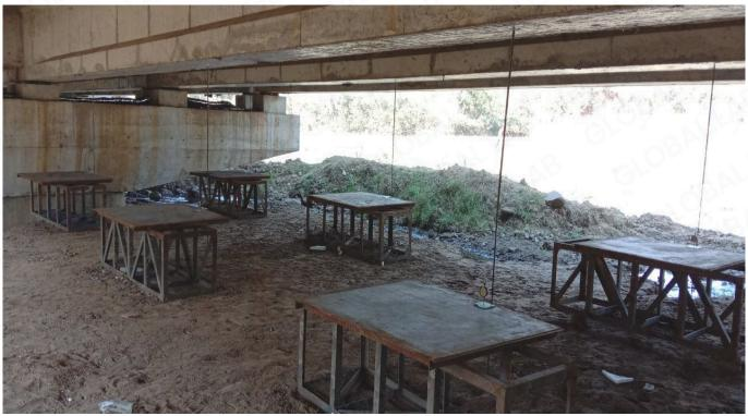
OBJECTIVE OF TEST: The proof load testing covers the testing of superstructures, excluding arches for evaluation of their flexural capacity. Testing for shear capacity of bridge superstructure is not considered. This test is not intended to assess the ultimate load-carrying capacity of the bridge superstructure.
