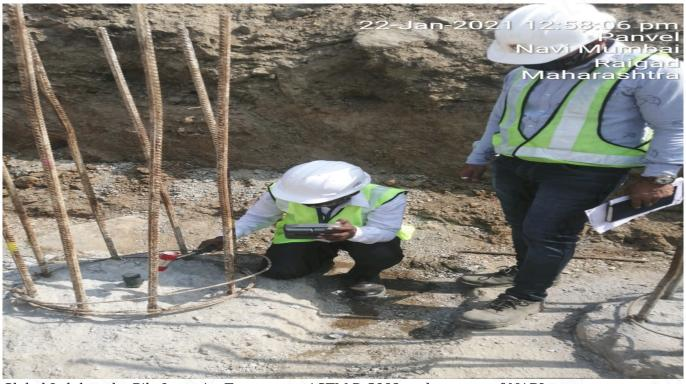
Global Lab has the Pile Integrity Test as per ASTM D 5882 under scope of NABL.
