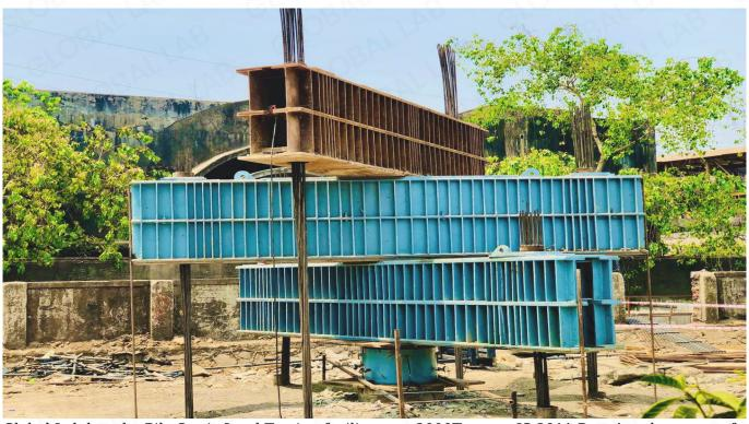
Global Lab has the Pile Static Load Testing facility upto 2000T as per IS 2911 Part-4 under scope of NABL.
