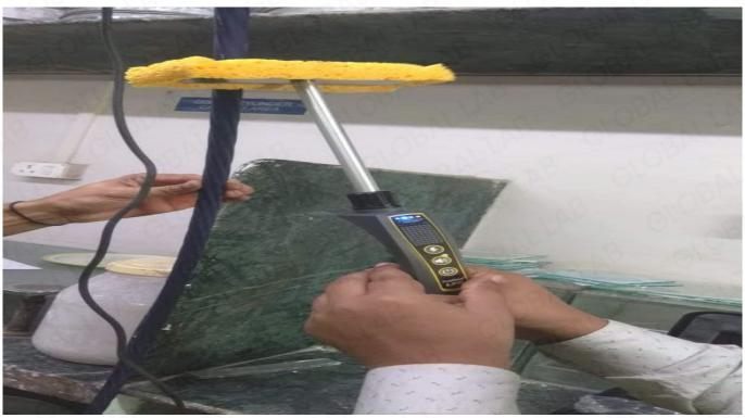
Global Lab has the facility to detect pin holes in the coating of bar and wires.
